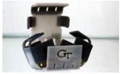
Here's something from SUTD! Our researchers and Georgia Tech have collaborated to design smart shapememory materials to demonstrate 4-D printing! This can result in complex structures capable of folding on their own, responding to external stimuli such as temperature, moisture or light to change to a preset shape. Potential applications of these materials may be in space structures, medical devices and robots! Way to go, SUTD!
